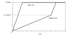
This fitting allows for a progressive pressurization of the installation and prevents the actuators from being hit hard in case of sudden pressure feeding of the previously vented circuit.
